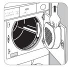
Do not be alarmed by the amount of fluff. It is not due to excessive wear caused by the dryer. All fabric loses fluff when drying but it goes un-noticed in the air. In a tumble dryer it simply collects in the filter. After a while, a whitish patina due to detergent residue on laundry forms on the filters. When this occurs, clean the filters with warm water using a brush. Remove the filter in the door opening as per picture (it can be positioned with the tooth facing to the left or to the right).
